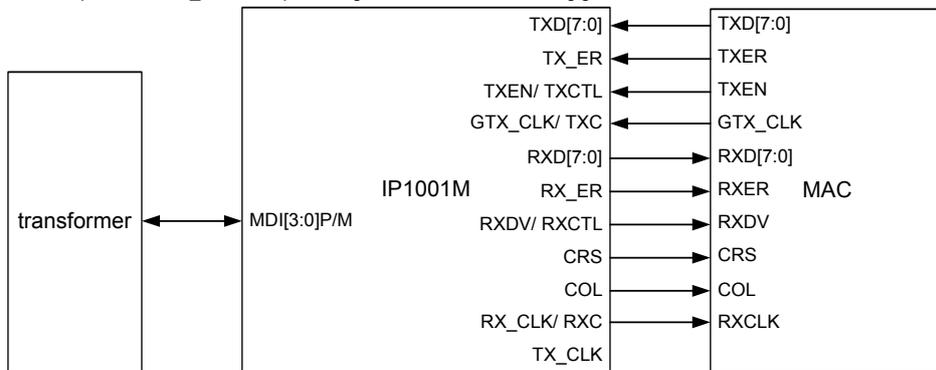
MII is active if pin 36 RGMII\_N/GMII is pulled high and IP1001 is linked at 100M, or 10M.
