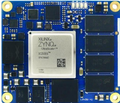
Figure 1-6 [MYC-CZU3EG/4EV CPU Module](#) Top-view
