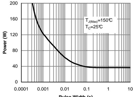
Figure 10: Single Pulse Power Rating Junction-to-Case (Note F)
