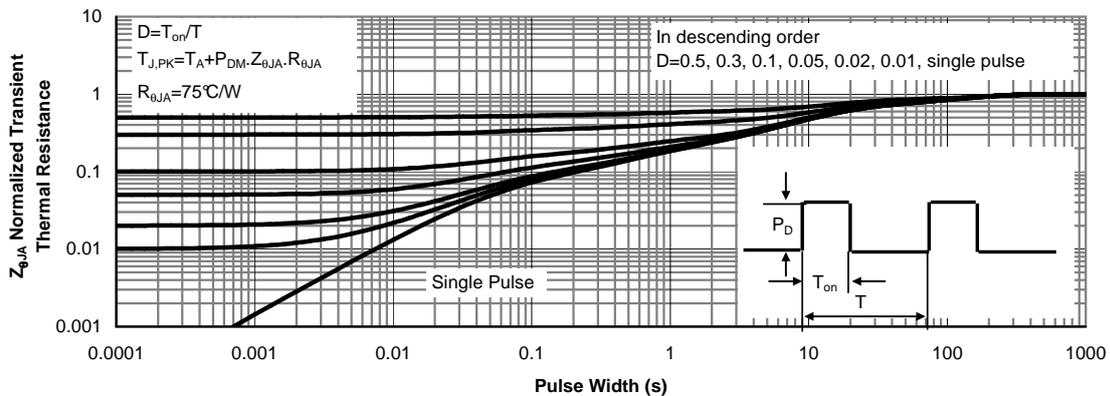
Figure 16: Normalized Maximum Transient Thermal Impedance (Note H)
