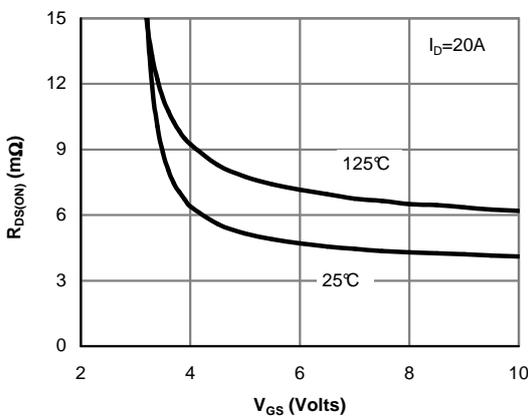
Figure 5: On-Resistance vs. Gate-Source Voltage (Note E)
