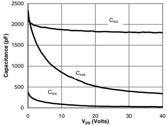
Figure 8: Capacitance Characteristics
