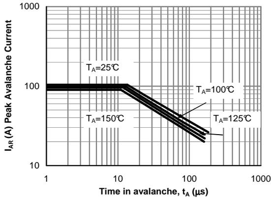
Figure 12: Single Pulse Avalanche capability (Note C)
