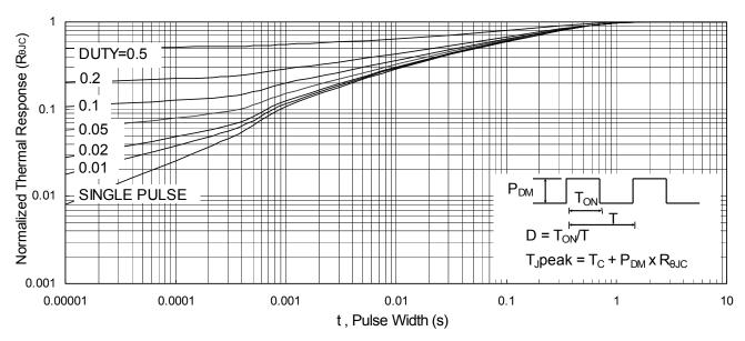
Fig.9 Normalized Maximum Transient Thermal Impedance
