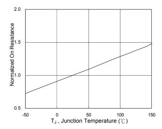
Fig.6 Normalized R<sub>DSON</sub> vs. T<sub>J</sub>
