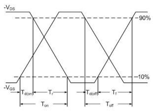
Fig.10 Switching Time Waveform
