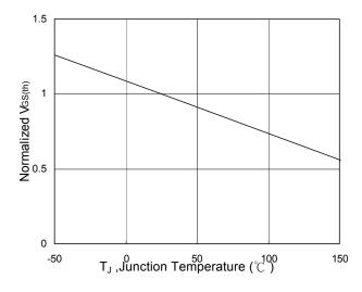
Fig.5 Normalized  $V_{\text{GS(th)}}$  vs.  $T_{\text{J}}$
