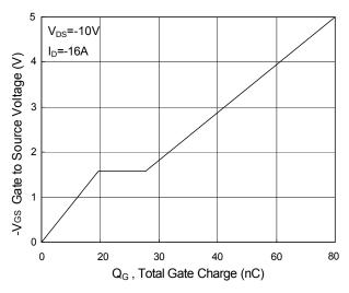
Fig.4 Gate-Charge Characteristics
