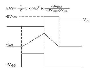
Fig.11 Unclamped Inductive Switching Waveform
