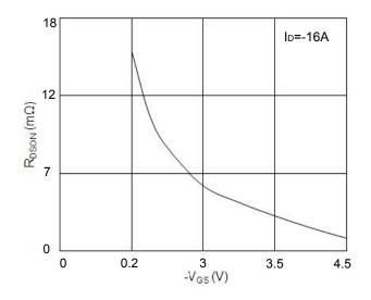
Fig.2 On-Resistance vs. G-S Voltage
