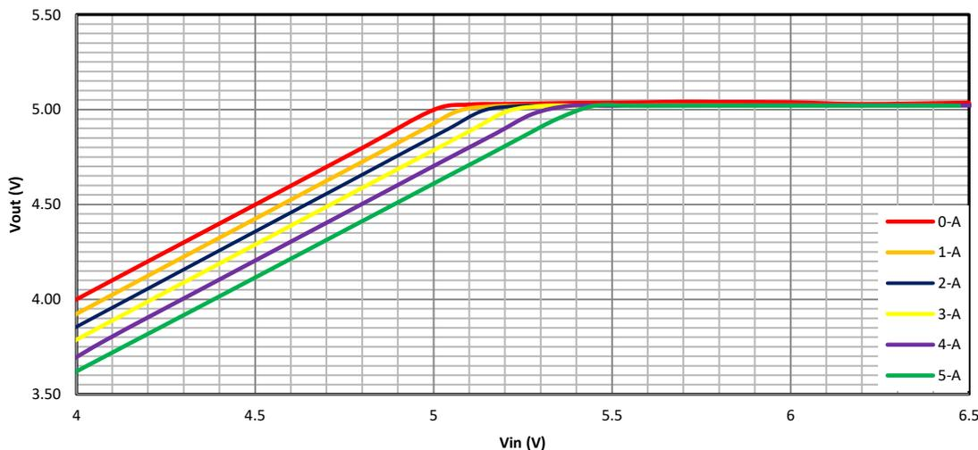
Figure 17. LDO Operation Characteristic (  $V_{out} = 5V$  )
