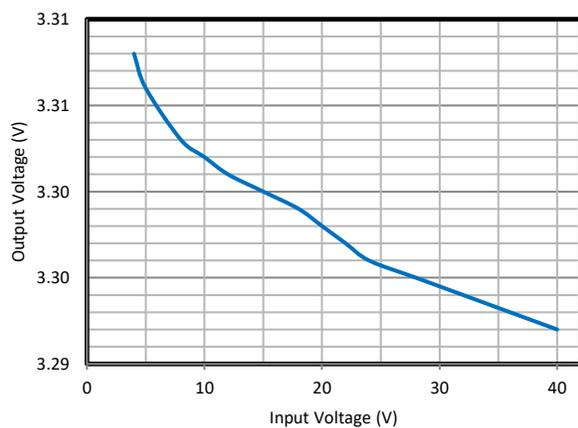
Figure 6. Line Regulation (Iout=5A)
