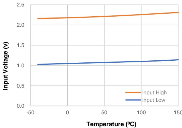
Figure 3. Input Threshold vs Temperature
