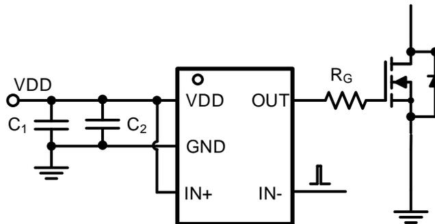
Figure 20. SCT51240 Inverting MOSFET Gate Drive Typical Application
