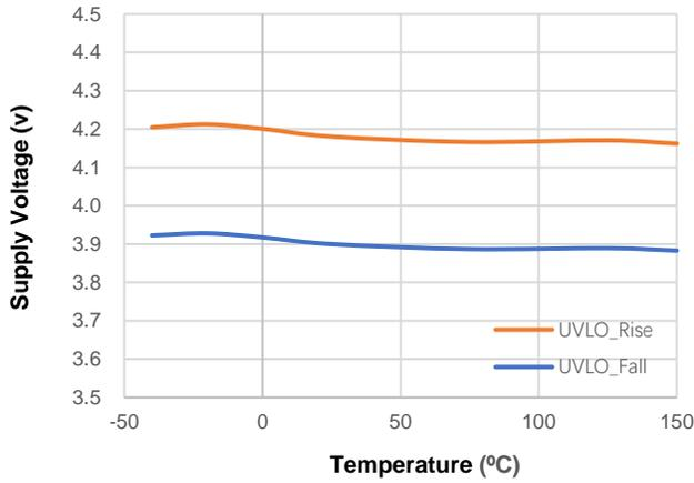
Figure 1. UVLO vs Temperature
