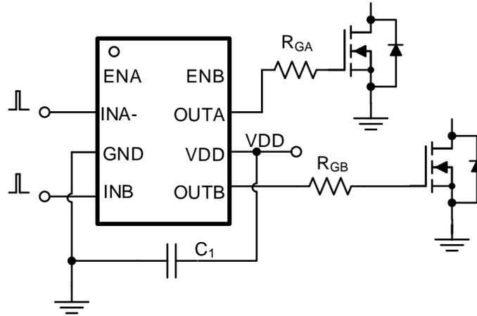
Figure 16. Dual Channel Driver Typical Application
