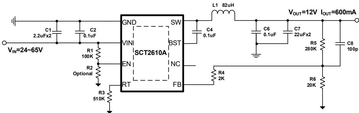
Figure 14. V<sub>OUT</sub>=12V, I<sub>OUT</sub>=0.6A Application Circuit
