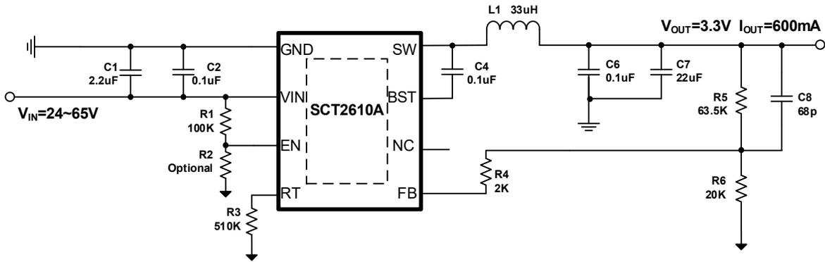
Figure 12. V<sub>OUT</sub>=3.3V, I<sub>OUT</sub>=0.6A Application Circuit
