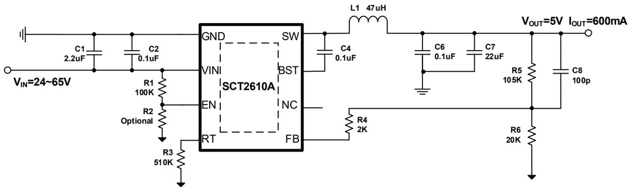
Figure 13. V<sub>OUT</sub>=5V, I<sub>OUT</sub>=0.6A Application Circuit
