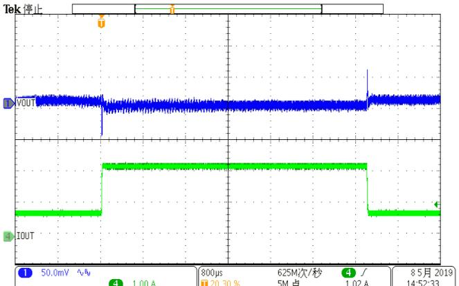
Figure 14. Load Transient
