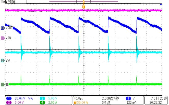
Figure 10. SW node Waveform and Output Ripple
