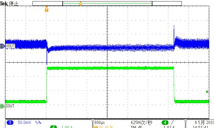
Figure 13. Load Transient
