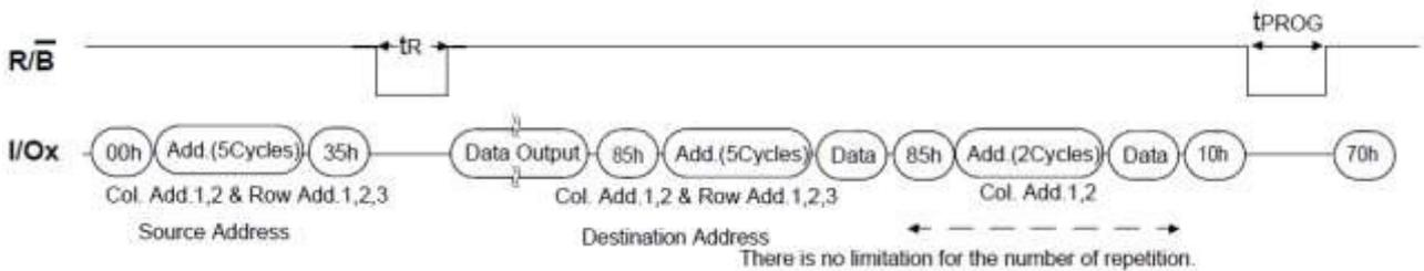
Figure 12 Copy-Back Program with Random Data Input Sequence
