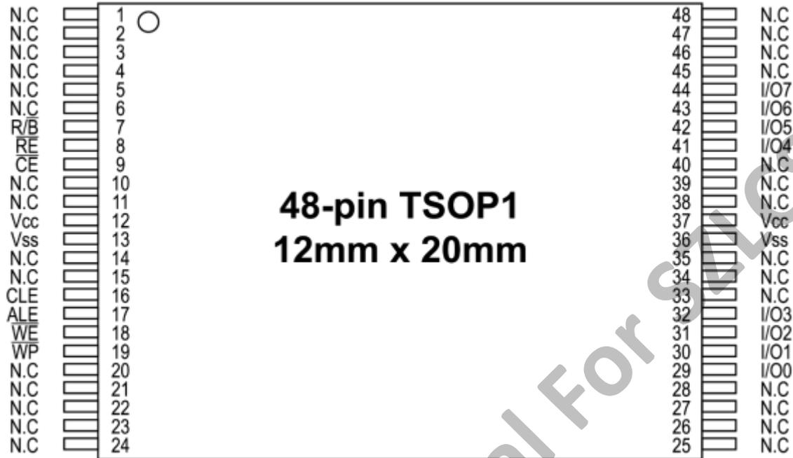
Figure 1 48 -Pin TSOP1 Contact x8 Device
