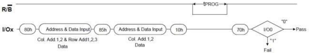
Figure 10 Program Operation with Random Data Input Sequence
