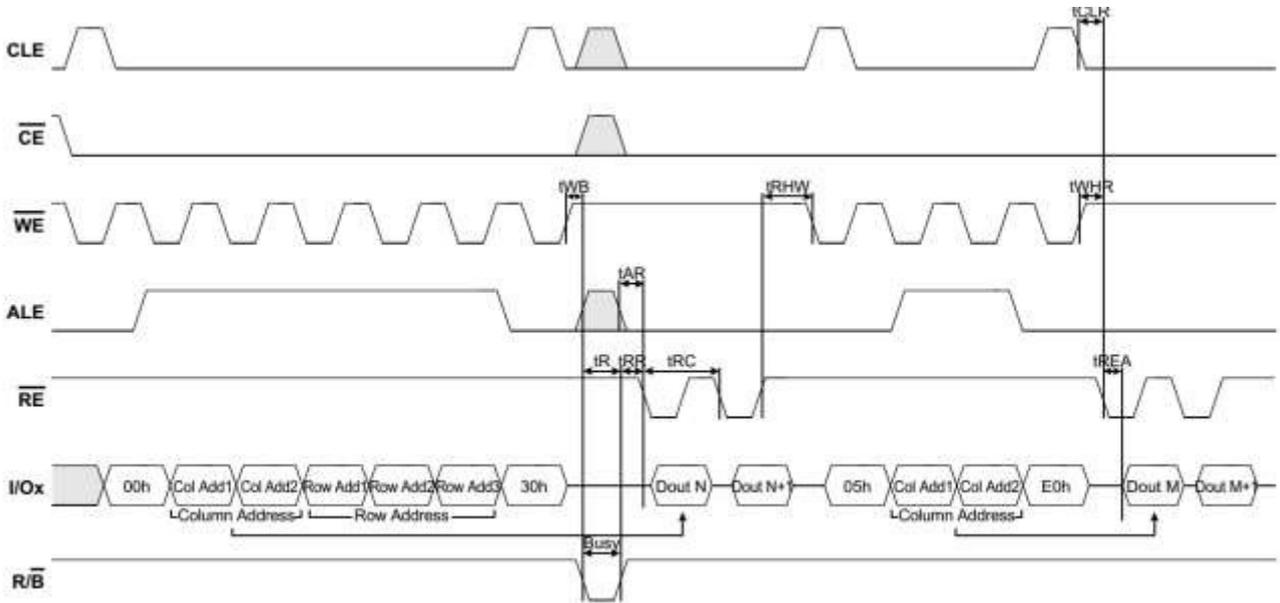
Figure 38 Random Data Output In a Page Operation
