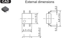
Terminal thickness = 0.15 General tolerance: ± 0.1
