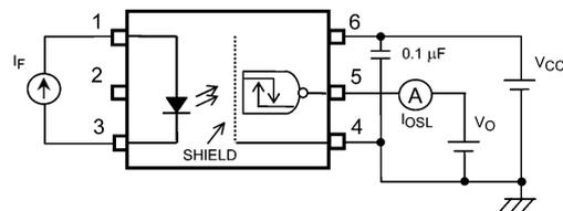
Fig. 13.1.5 IOSL Test Circuit
