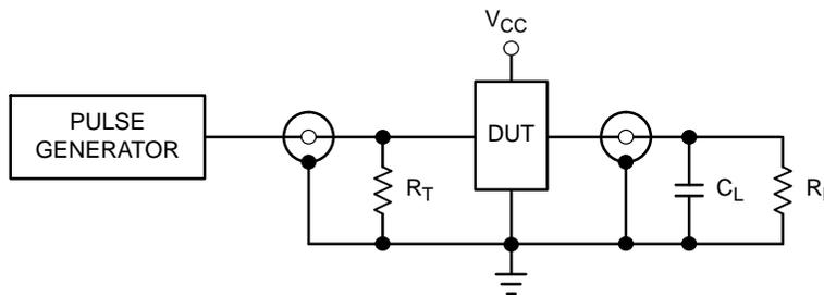
$C_L = 50 \text{ pF}$  at  $V_{CC} = 3.3 \pm 0.3 \text{ V}$  or equivalent (includes jig and probe capacitance)
