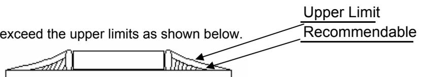
Accordingly increasing the solder volume, the mechanical stress to product is also increased. Exceeding solder volume may cause the failure of mechanical or electrical performance.
