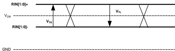
Figure 5. FPD-Link III Receiver DC  $V_{TH}/V_{TL}$  Definition
