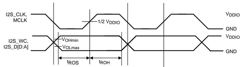
Figure 6. Output Data Valid (Setup and Hold) Times
