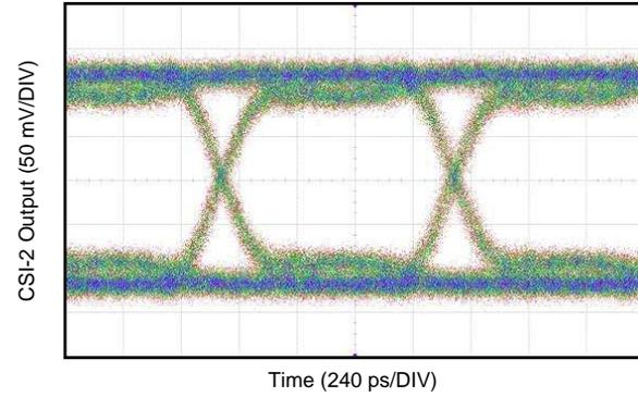
**Figure 43. CSI-2 Data Output at 1040 Mbps**
