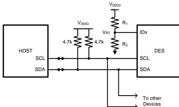
Figure 33. Serial Control Bus Connection
