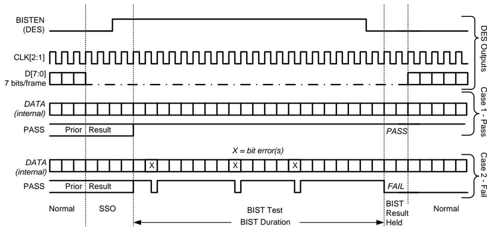
Figure 27. BIST Waveforms
