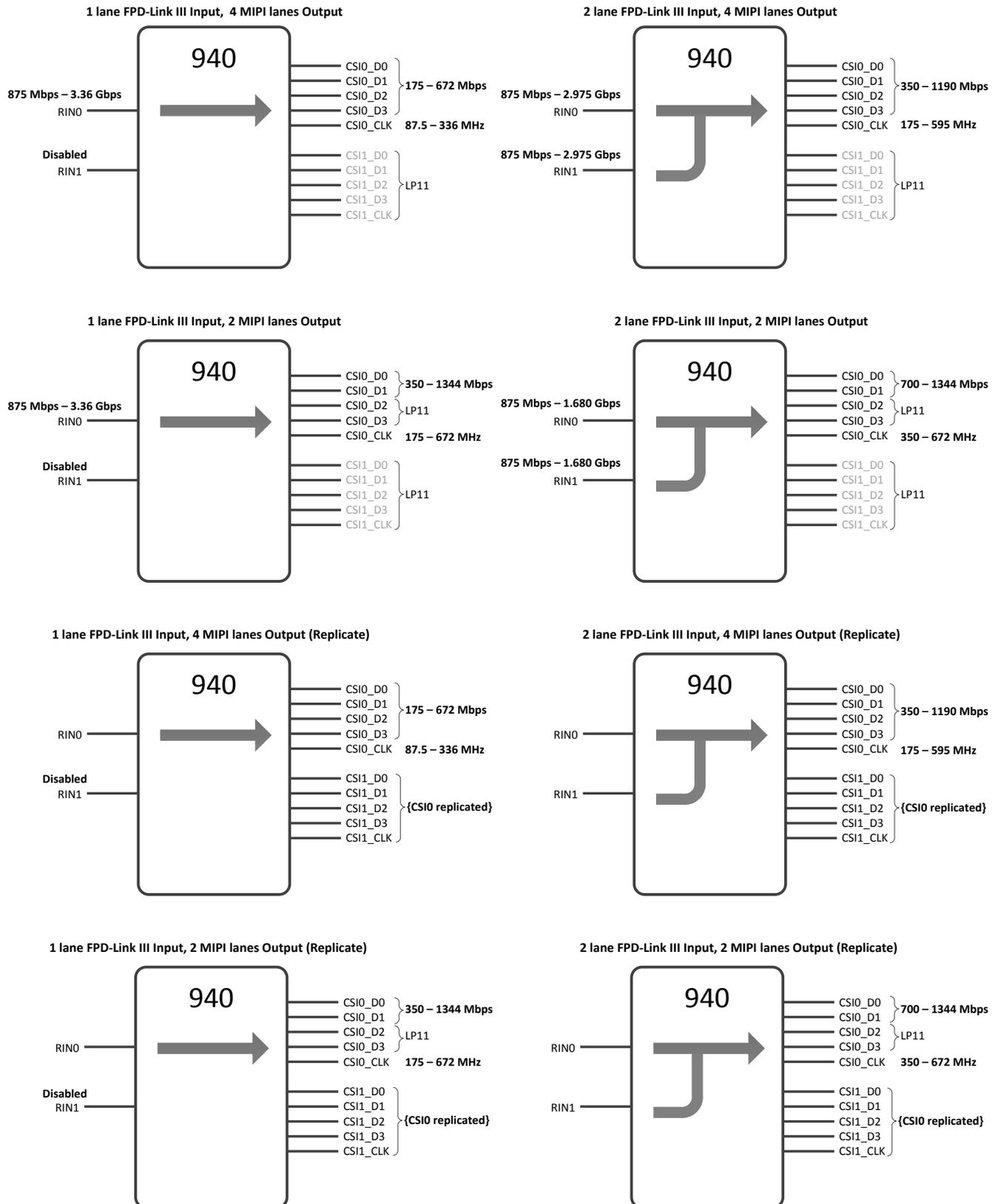
**Figure 28. Datapath Configurations**
