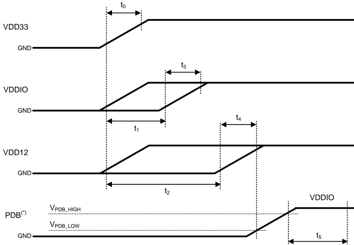
(\*) It is recommended to assert PDB (active High) with a microcontroller rather than an RC filter network to help ensure proper sequencing of PDB pin after settling of power supplies.
