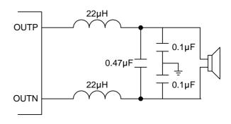
Figure 5. Typical LC output filter
