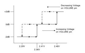
Figure 4. DC volume control operation
