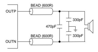
Figure 6. Typical ferrite chip bead output filter
