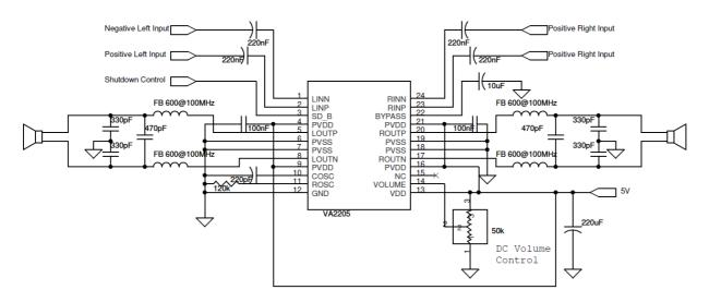
Figure 30. VA2205 with differential input configuration
