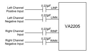
Figure 1. Differential stereo input configuration
