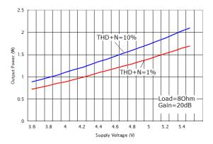
Figure 28. THD+N vs. Supply Voltage
