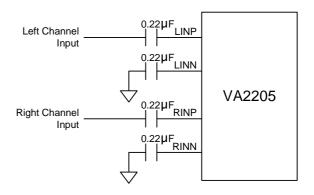
Figure 2. Single-ended stereo input application
