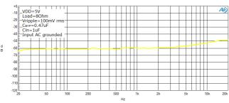
Figure 23. k<sub>SVR</sub> vs. Frequency
