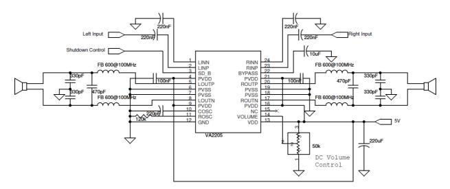
Figure 31. VA2205 with single-ended input configuration
