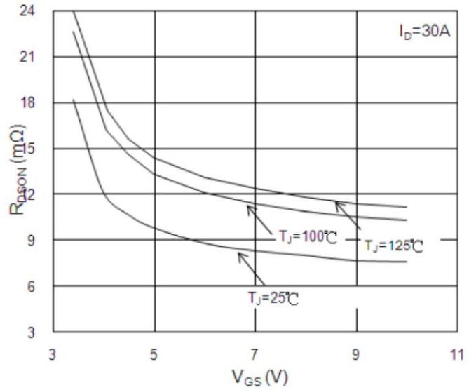
**Fig.2 On-Resistance vs. G-S Voltage**
