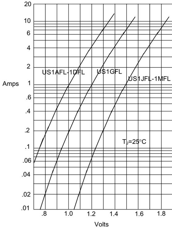
Instantaneous Forward Current - Amperes versus
