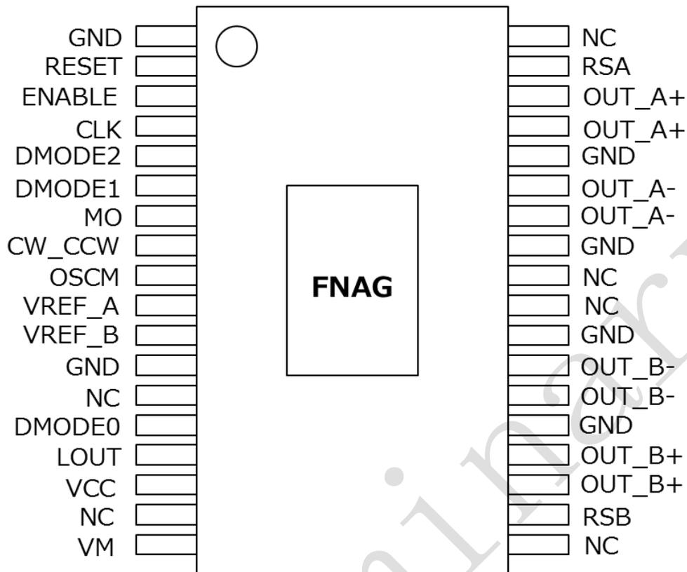
Please mount the exposed pad of the HSSOP package to heatsink .
