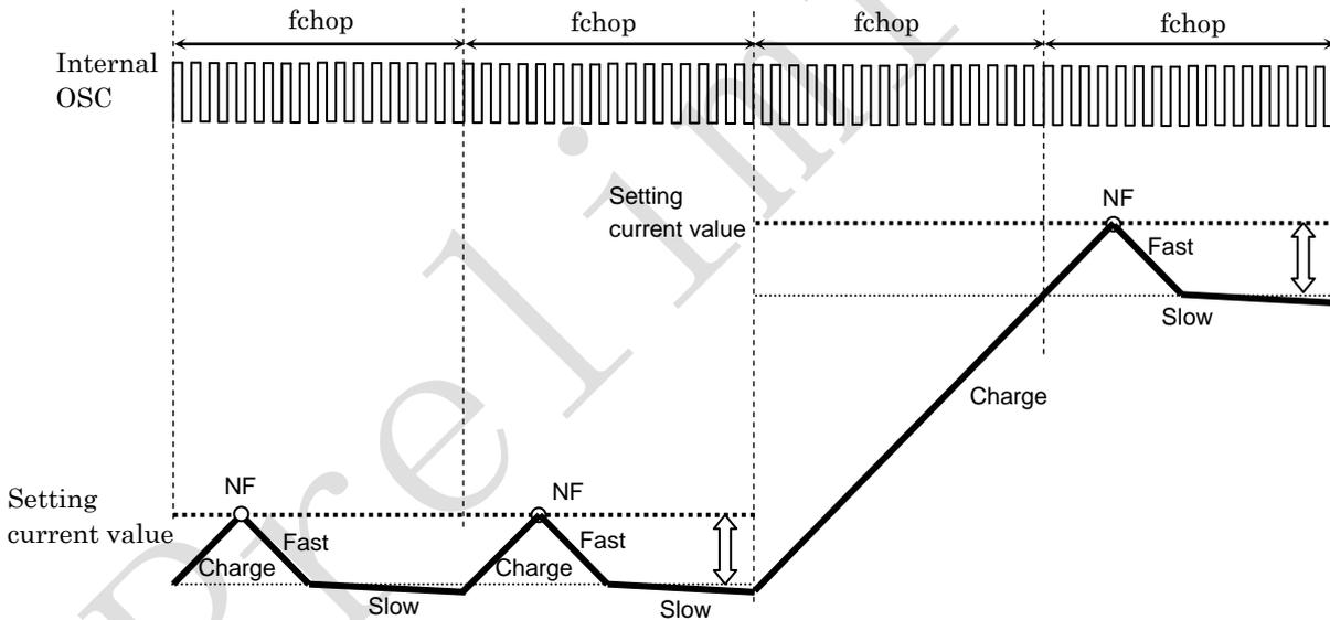
When the Charge period is longer than fchop cycle, the Charge period will be extended until the motor current reaches the NF threshold. Once the current reaches the next current step, then the sequence will go on to decay mode.
