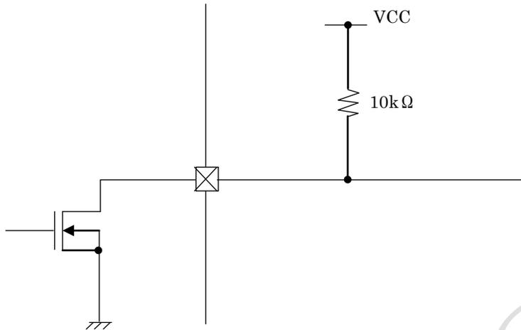
The LO is an open-drain output pin. LO pin needs to be pulled up to 3.3V/5.0V level for proper function. During regular operation, the LO pin level will stay High(VCC level). When error detection (TSD, ISD) is applied, the LO pin will show Low (GND) level.
