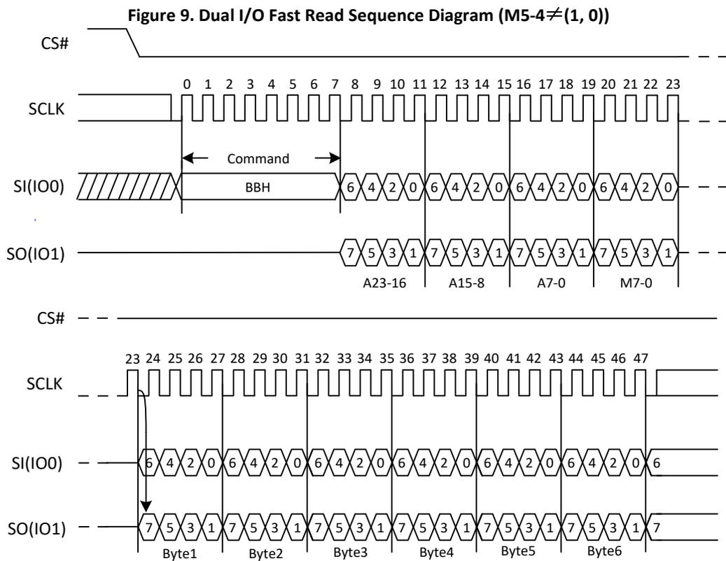
Figure 9a. Dual I/O Fast Read Sequence Diagram (M5-4= (1, 0))
