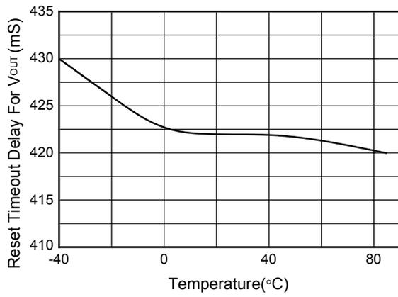
**Figure 10. t<sub>REC1</sub> vs. Temperature**
