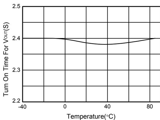
**Figure 8. t<sub>VON</sub> vs. Temperature**
