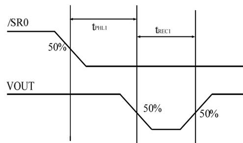
Figure 20. Reset Timing
