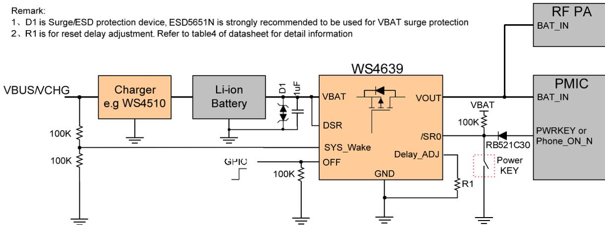
**Figure 1. Typical Application without power path system**
