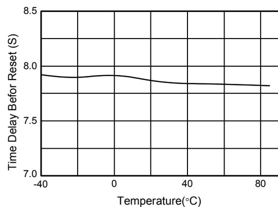
**Figure 9. t<sub>PHL1</sub> vs. Temperature**
