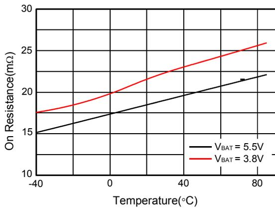
**Figure 6. R<sub>ON</sub> vs. Temperature**
