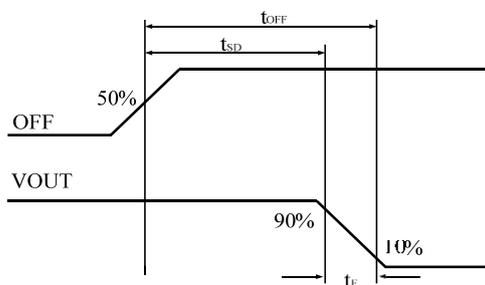
Figure 17. OFF vs. V<sub>OUT</sub>
