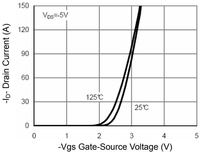
**Figure 2 Transfer Characteristics**
