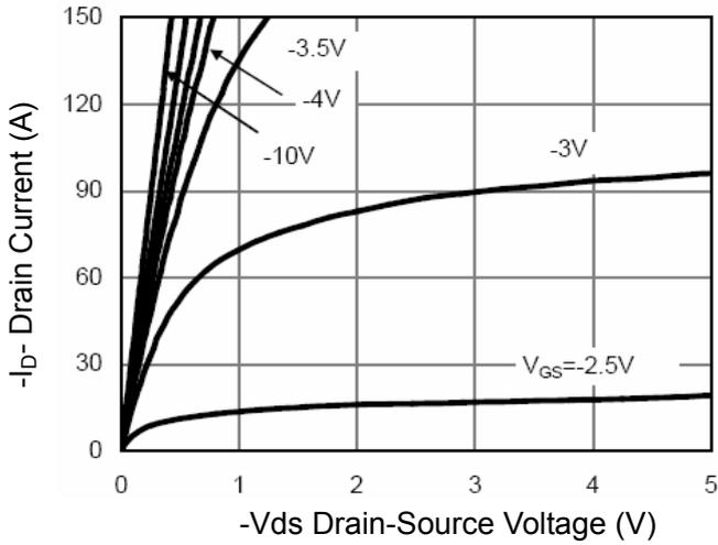
**Figure 1 Output Characteristics**
