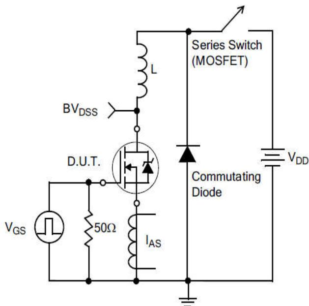
Figure17. Unclamped Inductive Switching Test Circuit
