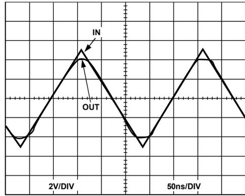
Figure 33. Input Overdrive Recovery, Gain = +1
