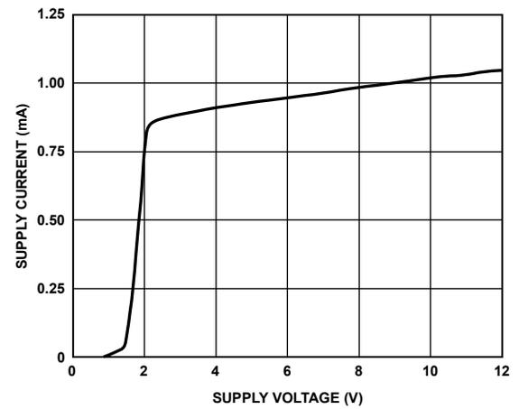
Figure 41. AD8038 Supply Current vs. Supply Voltage
