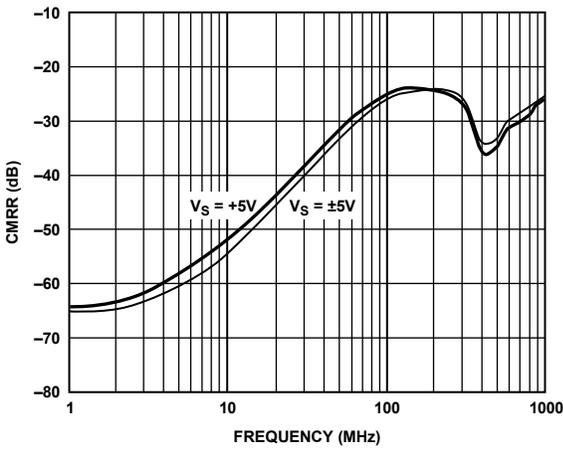
Figure 37. CMRR vs. Frequency,  $V_{IN} = 1\text{ V p-p}$
