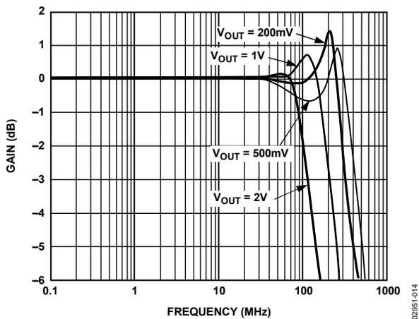
Figure 14. Frequency Response for Various Output Voltage Levels
