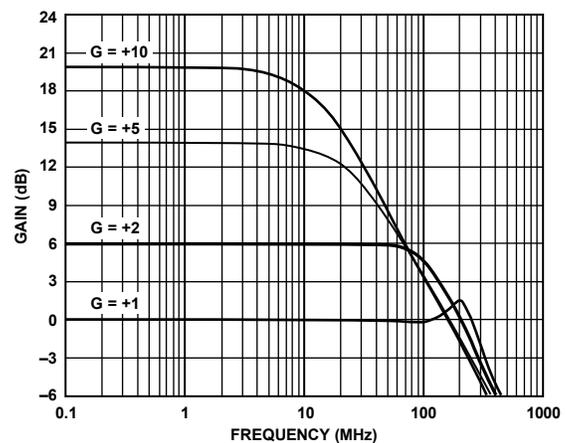
Figure 4. Small Signal Frequency Response for Various Gains,
