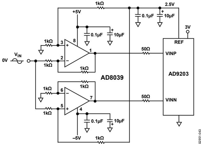
Figure 43. Schematic to Drive AD9203 with the AD8039
