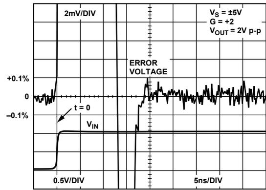
Figure 35. 0.1% Settling Time  $V_{OUT} = 2V$  p-p
