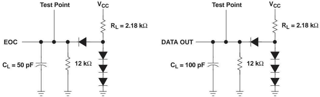
**Figure 2. Load Circuits**
