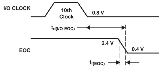
**Figure 7. I/O CLOCK and EOC Voltage Waveforms**
