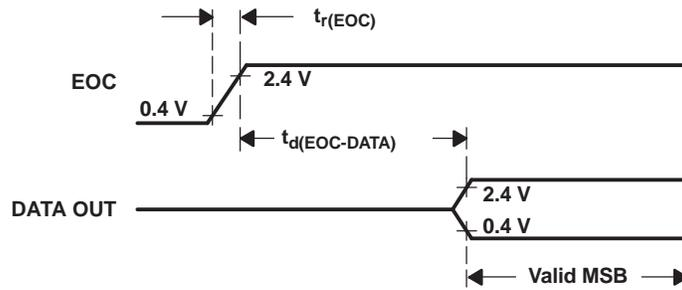
**Figure 8. EOC and DATA OUT Voltage Waveforms**
