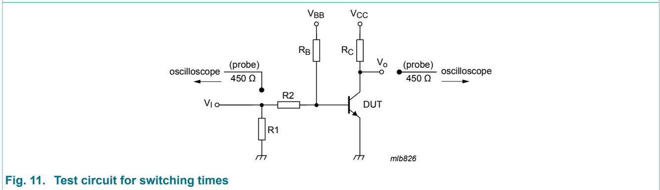
Fig. 11. Test circuit for switching times
