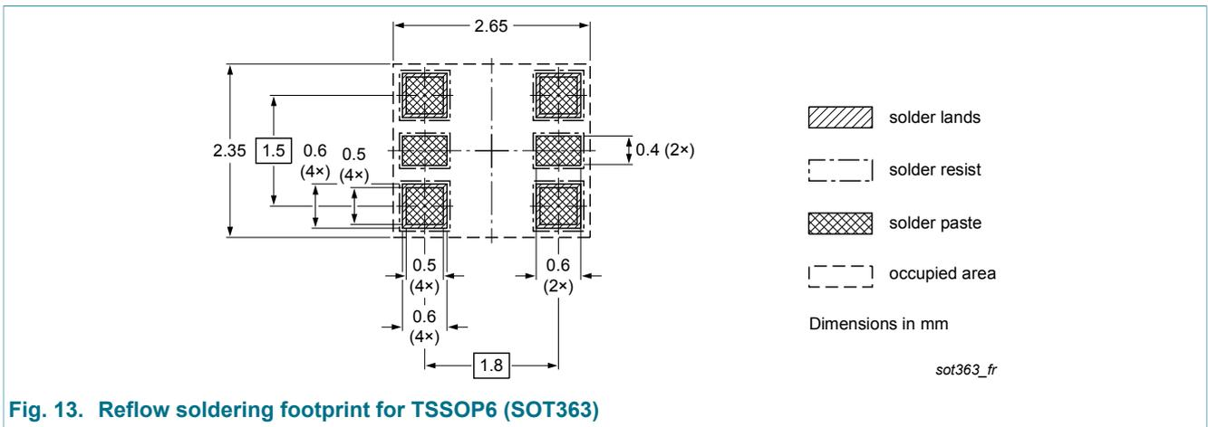
Fig. 13. Reflow soldering footprint for TSSOP6 (SOT363)
