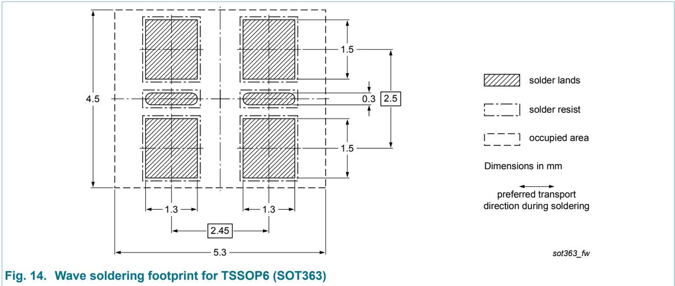
Fig. 14. Wave soldering footprint for TSSOP6 (SOT363)
